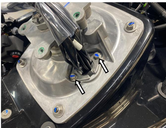
Remove center access cover (A) just below steering base plate.
