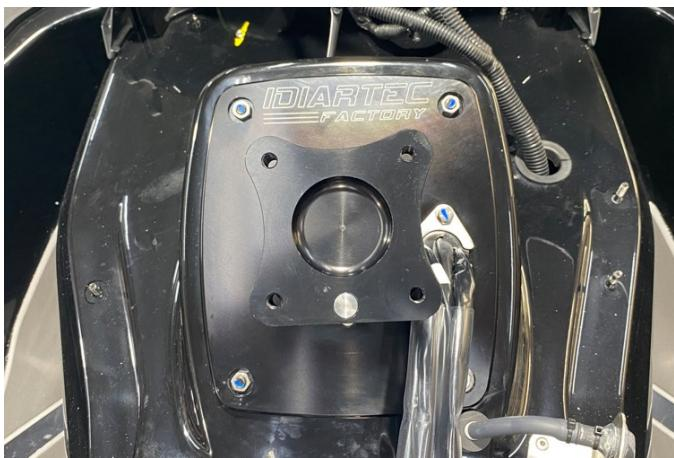
Install supplied steering head onto steering shaft and secure with supplied M8 bolts (4). *R logo faces forward!* **NOTE: Apply red Loctite to bolts. Torque to 15ft•lb (20 N•m).**
