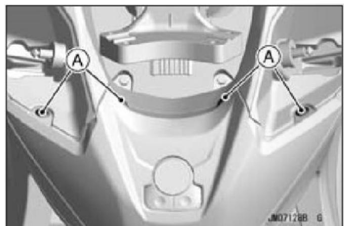
Remove console control cover (A) by carefully lifting front edge over control knob. Then, while pushing down at center to clear hooks (B), pull bottom edge out.
